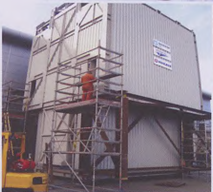
70t Pollution control unit for the Enasco 101 - manufactured & tested at our Links Place facility
