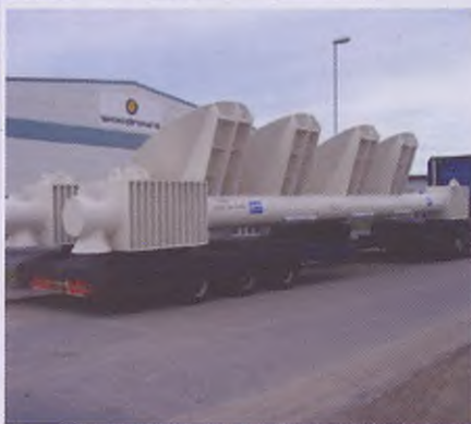
1 of 2 conductor guide frames manufactured for the Magnus - 100t each
